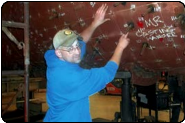
Mike pointing out one of the squares and bolt needing x-rayed and documented for the boiler rebuild.
